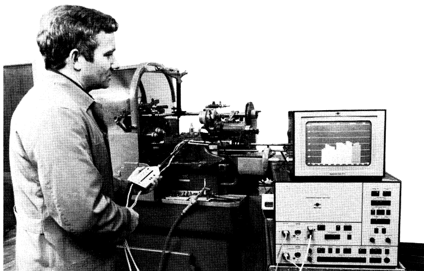
Fig. 30. Continuous sweep method for locating sound sources on a small lathe. As the median plane of the probe is swept past the source, i.e. the pulley and gear housing, the mid-frequencies of the displayed intensity spectrum change in brightness
